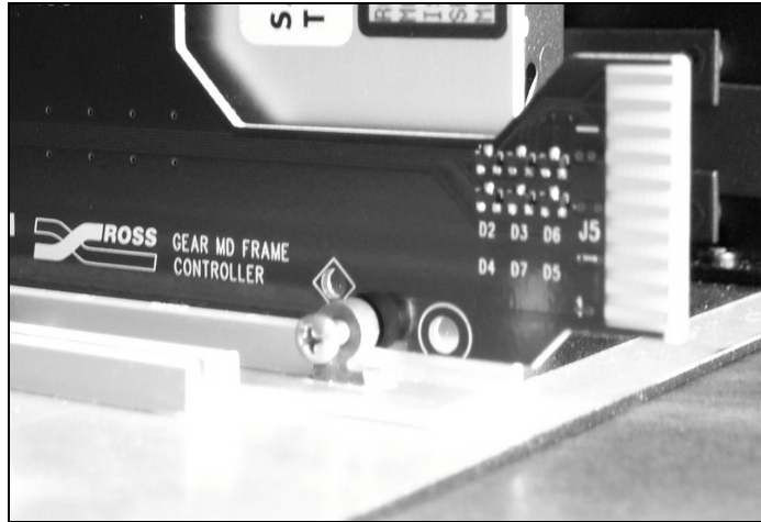
Figure 11. MFC-8310 Fan Controller Card and Unscrewed Retaining Screw
